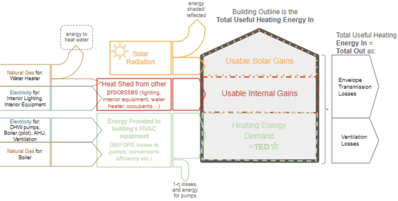
Figure 6. Building energy sub-model schematic.
