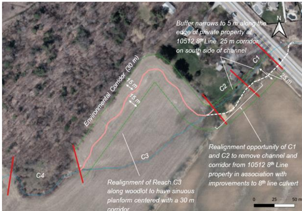
Figure 4.1: Plan view of the proposed realignment of reach C3, centered along a 30 m-wide environmental corridor contiguous with an existing woodlot.
