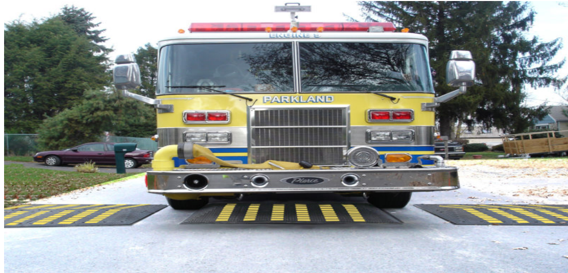
Fire Department Truck driving over speed cushion
