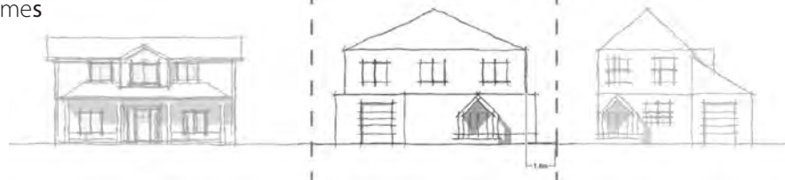
Sketches of proposed interior side yard setback for homes of different heights.
