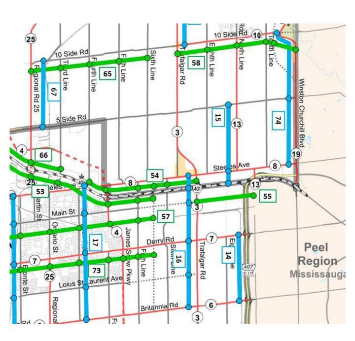
2031 TMP Network – With 5 ½ Line Test Scenario PM Peak Hour Total Vehicle Volume
