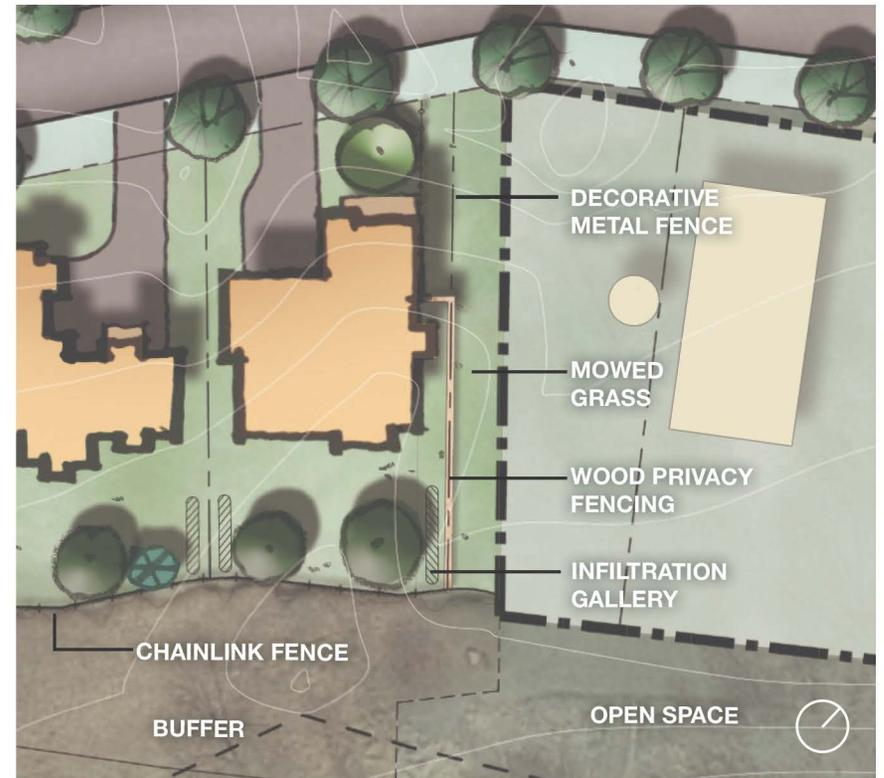
Figure 4.3 - Conceptual Landscape Plan of the 5m Stormwater Drainage Block
