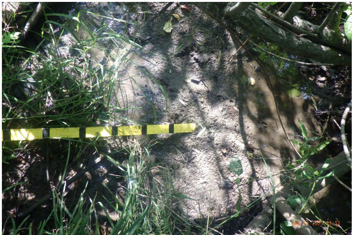
The bed and bank substrate in Reach N-2-D was primarily comprised of clay- and silt-textured materials.
