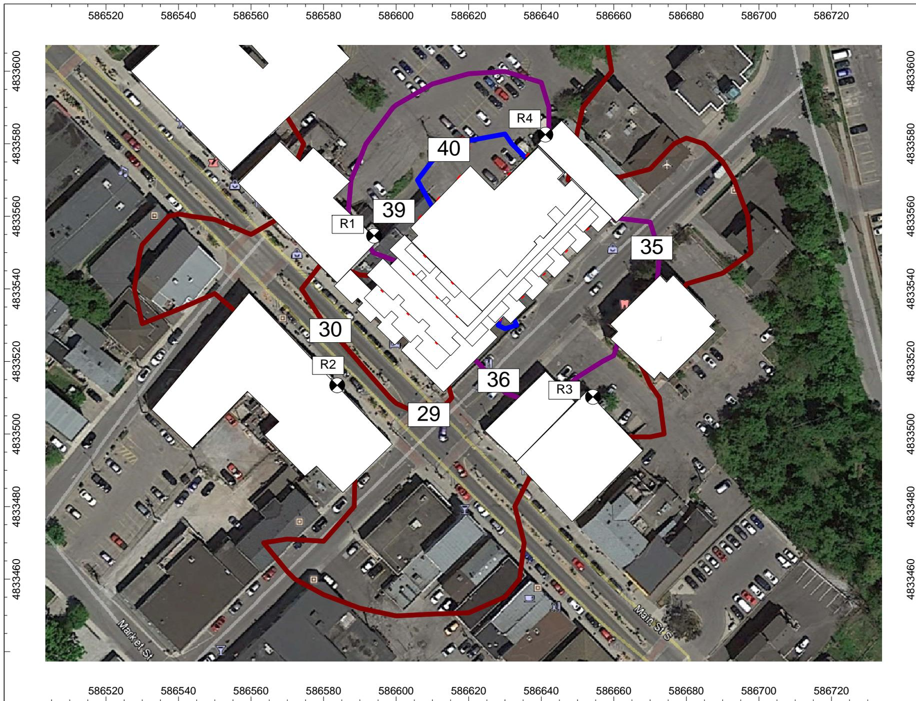
Figure 3: Daytime Sound Level Contours, without Mitigation, at 4.5 m Height
