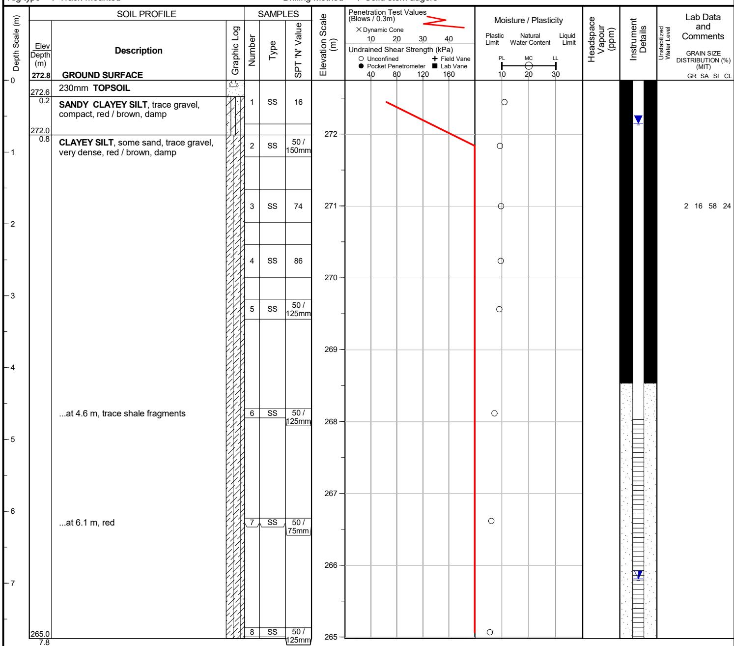
Borehole was dry and open upon completion of drilling.
