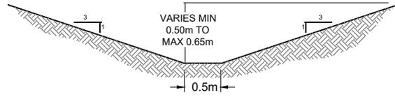
**TYPICAL FLAT BOTTOM PHASE 2 OUTLET SWALE**
