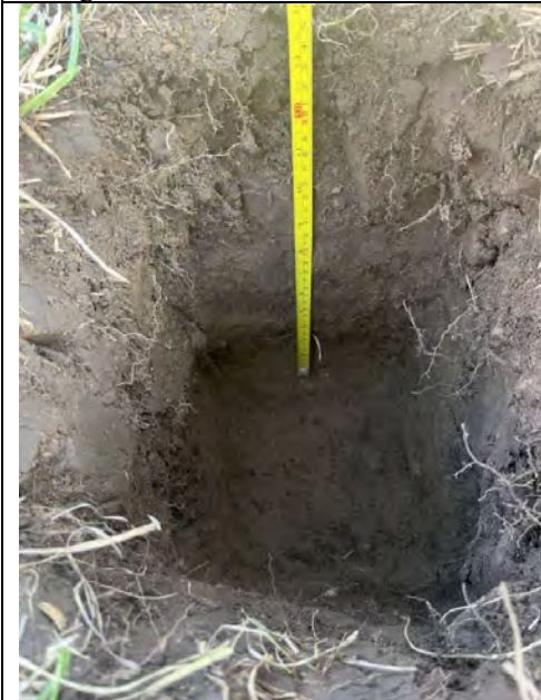
Image 7: Example of undisturbed test pit.
