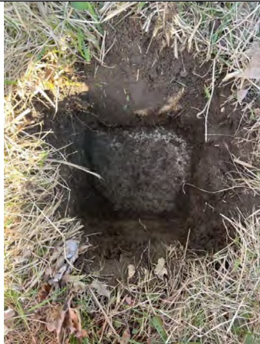
Image 6: Example of disturbed test pit - sloping concrete within test pit.
