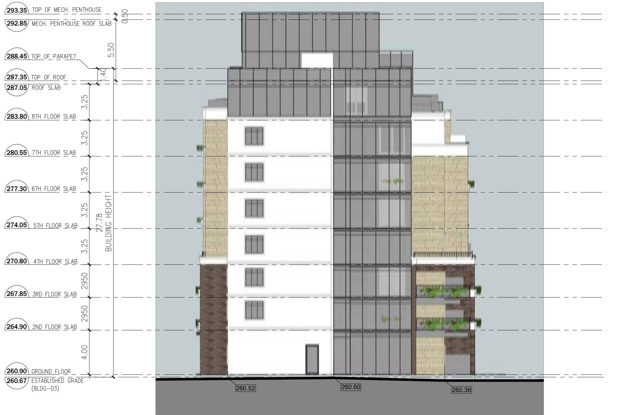
BUILDING - 3 _ SOUTH ELEVATION _ SCALE 1:200
